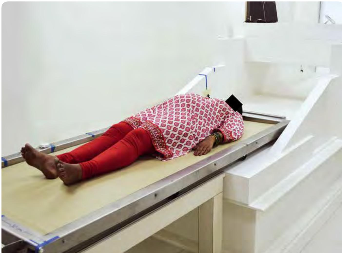
FIGURE 1: Shadow shield whole-body potassium counter facility at St John's Research Institute, Bangalore, India
